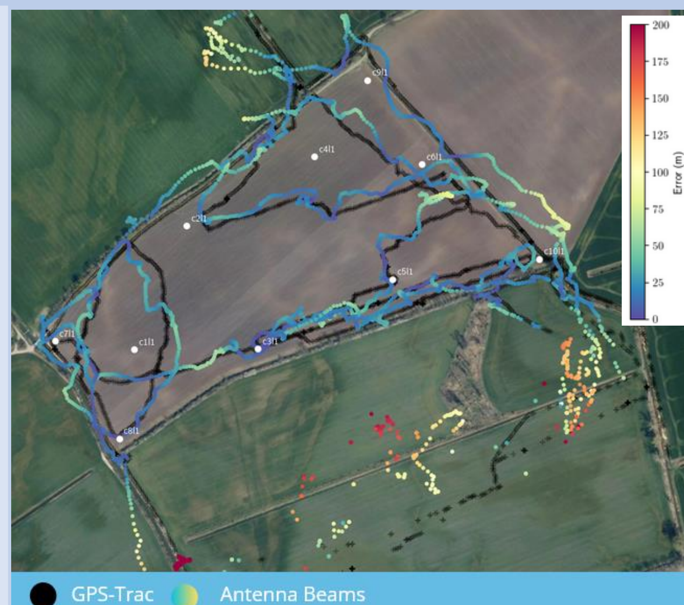
Fig. 8: Comparison of GPS track and position calculated by the automatic telemetry unit with tRackIT directional antennas [3] .
