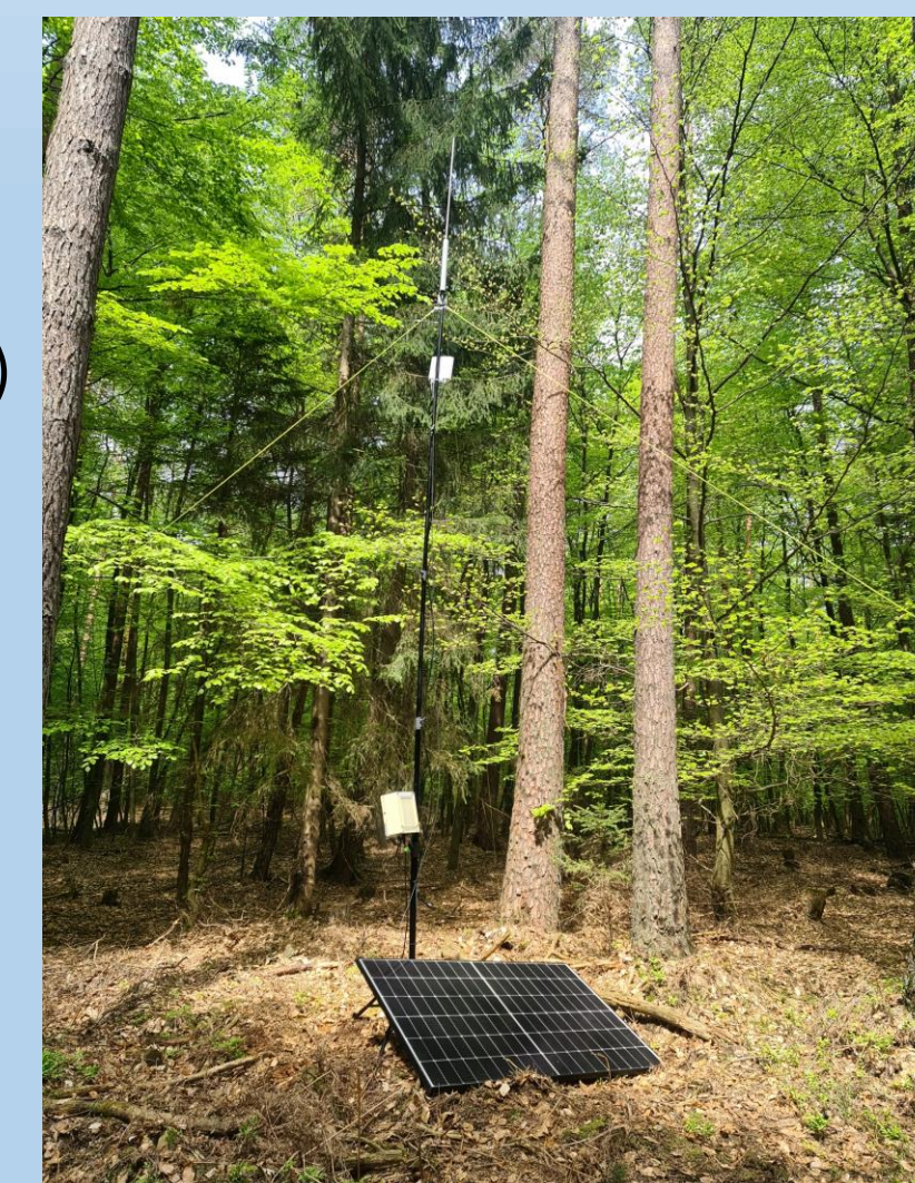
Fig. 1: Autonomous telemetry unit with an omnidirectional antenna from tRackIT Systems in a mixed deciduous forest clearing. The unit was placed as close as possible to the planned wind turbine site to obtain precise information on the foraging behavior of the animals within a 400 m radius of this point.
